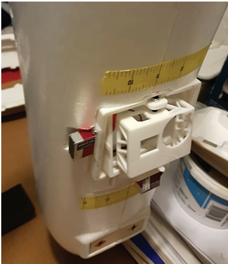
Gimbal installed in fuselage of our competition aircraft
